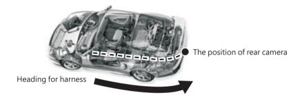
1.3 Connect the rear trigger with reversing light signal in the trunk.
