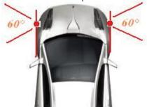
2.2 Drill a camera mounting hole with ø20mm on the left and right corner of front bumper. Assemble camera and harness temporarily until the all system install completely. Fix the camera after confirm the image and signal source are correct in last step. Please keep camera toward upside with triangle sign. (The triangle is on the side
